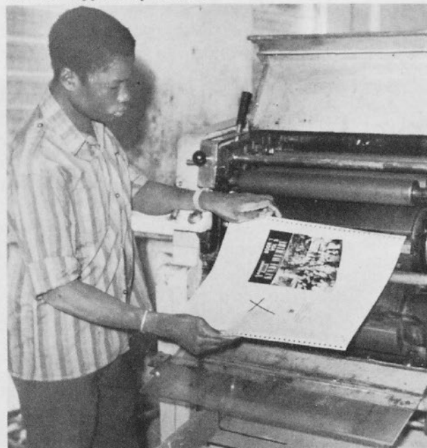
A national inserts plate into the offset press. These plates are also supplied by BGMC.
