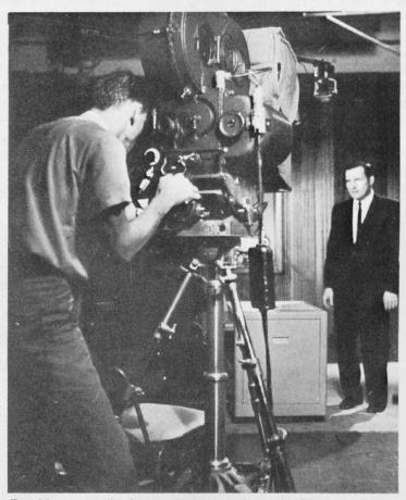
For 35 mm. productions, equipment such as the Mitchell 35 mm. motion-picture camera shown here is readily available on a rental basis. In this scene a professional teleprompter unit is being used for direct on-camera shooting.
