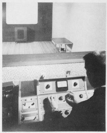
Mixing of the various sound tracks is done on the Magnasync Master Control Audio Console. As many as six separate tracks can be simultaneously mixed onto the 16 mm. composite master. Picture work print is also interlocked with the system to permit simultaneous picture viewing with the sound-dubbing operation. (Tract equalization can also be effected by means of the equalization loss pad.)
