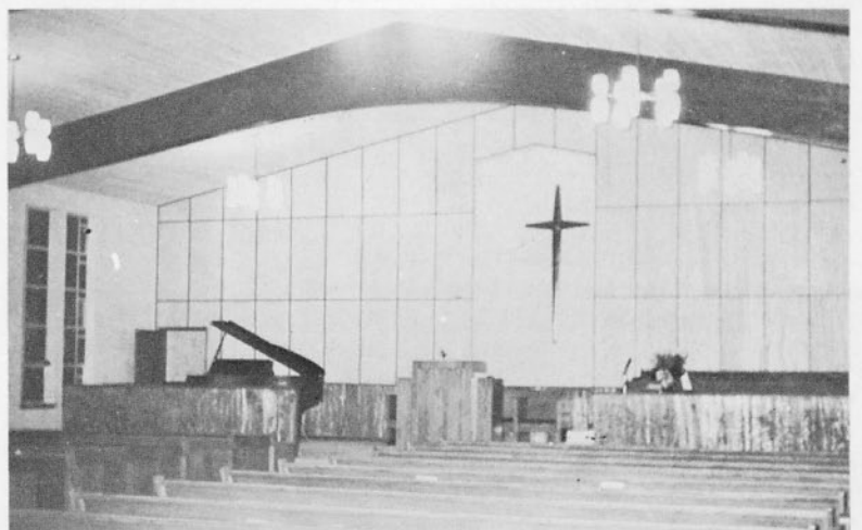
The sanctuary seats 325 and features open beam construction, ripplewood paneling on the platform, walnut pews and trim.
